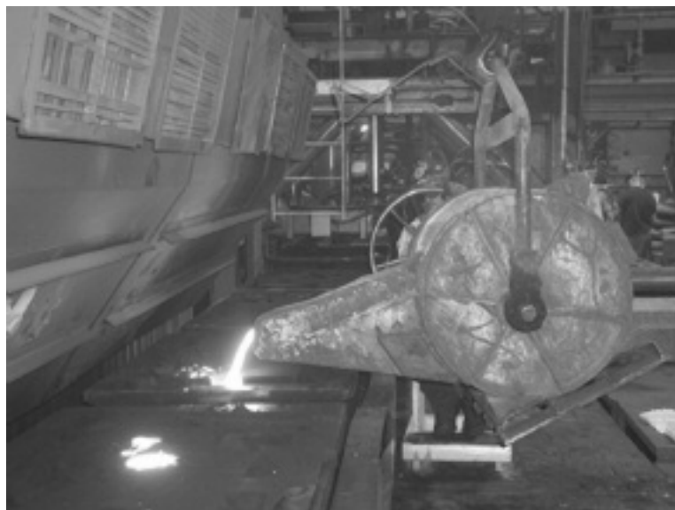
Figure 17—Rotating Wheel-Type Machine for Fittings Production.
