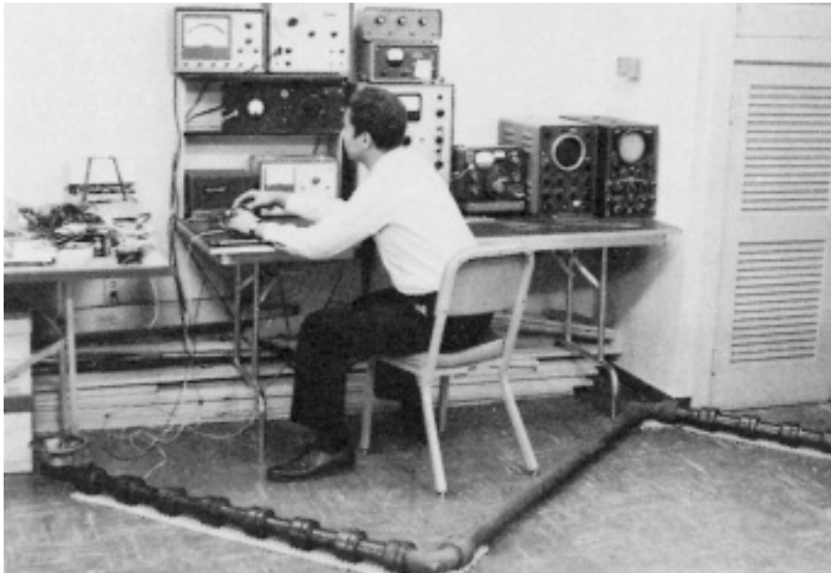
Figure 3—A “Z” Rig Being Tested for Acoustical Characteristics (Cast Iron with Neoprene Compression Gaskets).
