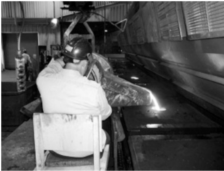
Figure 14—Hand-Pouring of Cast Iron Soil Pipe Fittings.
