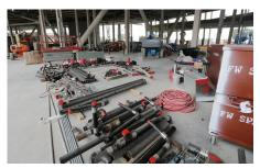
"By using cast iron piping materials along with the Husky couplings, we are able to air test the system at our manufacturing facility and then transport the complete plumbing systems to the building site without the worry that there would be joint failure.
